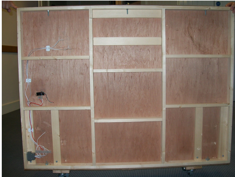
Figure 8: Wiring Runs (Right side)
